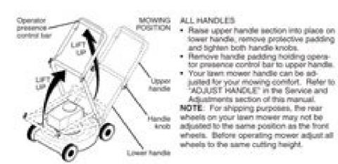
lower handle, remove protective padding and tighten both handle knobs.
